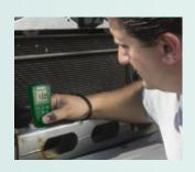
Extech's CG104 offers a quick, one-handed operation, non-destructive measurement of the thickness of ferrous and non-ferrous substrates. Its unique reversible display allows you to take readings in challenging angles of area being measured.
