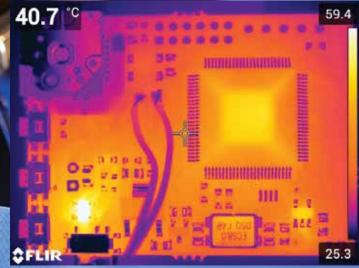
With the sensitivity to detect temperature differences of less than 0.03°C, the FLIR T530/T540 allow you to find hidden design flaws and track small thermal gradients. These cameras offer a wide temperature range for quantifying heat generation and thermal dissipation up to 1500°C (T540). Measurements are accurate to  $\pm 2\%$ , promoting quality assurance and factory acceptance of printed circuit boards and other products.
