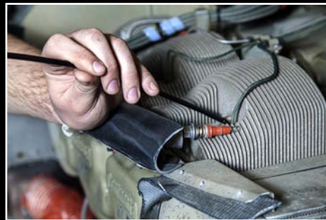
Inspecting cylinder in aircraft motor with VSA2-1M
